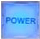
The main power switch for the Solice mixer is isolated along the right hand edge of the mixer. It is the top most large, square push button switches. This switch is a latching type. Press it once to turn on the mixer and press it again to turn off the mixer. When the mixer is powered on, this switch will be lit blue.
