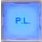
The Solice mixer is equipped with a private line function which allows the mixer operator to speak to the two boom operators at will. When this momentary switch is pressed, the slate microphone is routed to the two boom operator's headphones. Thus the mixer can talk to the two boom operators.
