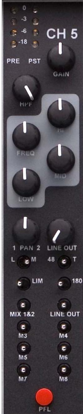
**CHANNEL METERS, PRE-FADER and POST-FADER**
