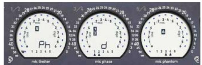
In the example above, the 'Ph d' phone routing indicates: track 5 goes to the left ear, track 1 and track 2 go to the center (both ears) and track 6 goes to the right ear. With the [SoloMixPan] slider pulled toward the operator side, pressure on the [routing] button instantly displays the current monitor configuration.
