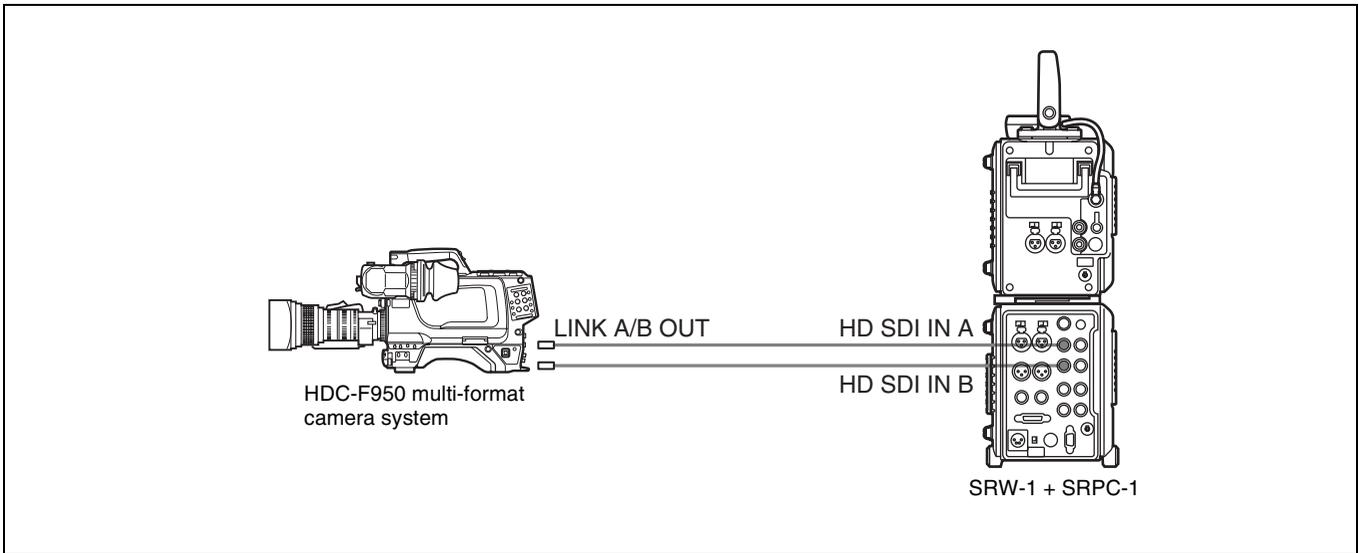
**To record the output of 2 camera systems as 4:2:2 DUAL STREAM**
