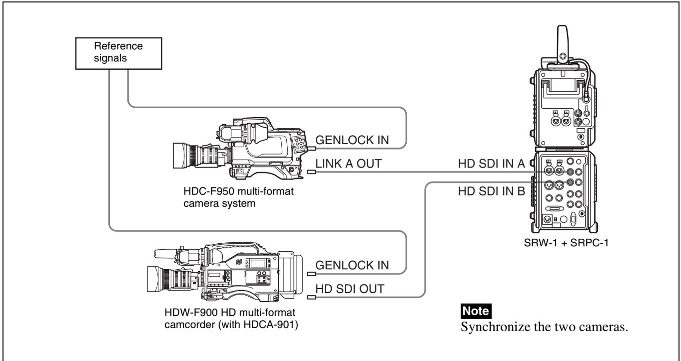
**To record 4:2:2 or 4:4:4 signals using optical-fiber cable**
