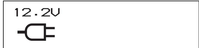
Note that this mark does not reflect the actual type of power being used, but reflects the settings of the following menu items.
