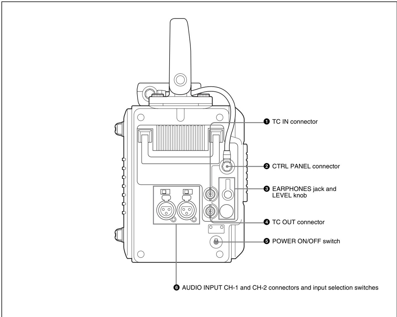
**1 TC IN (timecode input) connector (BNC type)**
