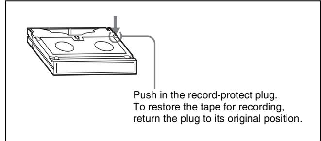
When a cassette with the plug in this position is inserted into the recorder, the REC INHI indicator lights up on the control panel display and recording will not start, even if you press the REC and PLAY buttons.
