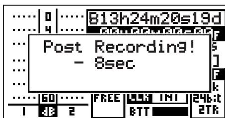
Press the [REC] key while "Post Recording!" is shown as above.
