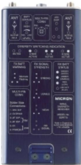
The SDR770 offers excellent standards of RF performance - multiple RF stages give outstanding sensitivity and selectivity, and the digitally controlled PLL offers optimum mobile operation. The unique noise reduction system provides trouble-free operation in low RF signal situations, even in hostile RF environments.
