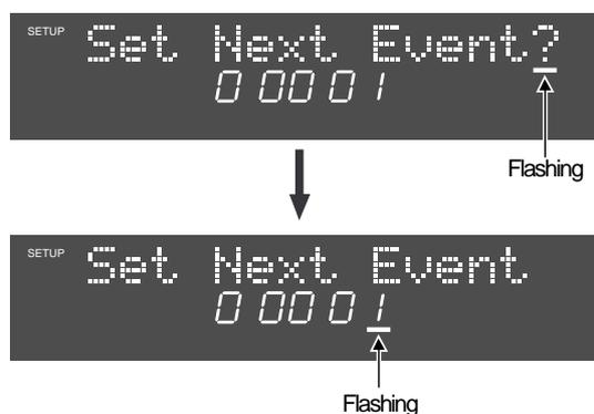
3. Input a desired number by the JOG dial (or 10 key) and press the [ENTER/YES] key.
