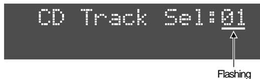
2. Input a desired track number by rotating the JOG dial or 10 key and press the [ENTER/YES] key.
