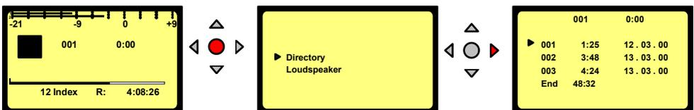
By using the **“UP”**, **“DOWN”**, **“LEFT”**, **“RIGHT ARROW”** keys ( 9, 11, 10, 12), once **“DIRECTORY”** has been selected, it becomes possible to scroll vertically and horizontally to view all the recorded indexes and their specifications.
