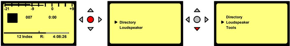
By pushing the “**CENTER**” key (13), the machine gives access to the “**DIRECTORY**”, “**LOUDSPEAKER**”, “**TOOLS**”, “**TEMPLATES**”, “**SETTINGS**” etc. sub-menus. Using the “**ARROW**” keys (9 to 12), you navigate between those sub-menus. To move back to the initial display, press the “**LEFT ARROW**” key (10) (except in the “**DIRECTORY**” where “**CENTER**” key (13) needs to be pressed first to return to the sub-menus).
