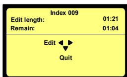
If the remaining time on the card is shorter than the selected index length, a new window will appear but without the “SAVE” possibility. It is up to the user if he thinks that once the index is edited, the size will be smaller than the remaining time. In this case the “EDIT” can be selected.
